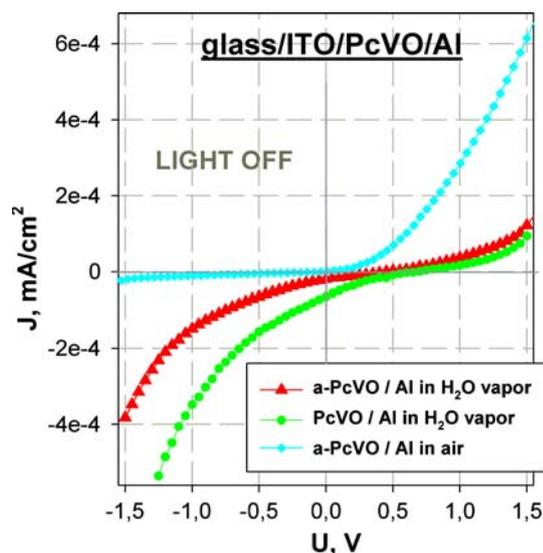
**Fig. 3**  $J$ - $V$  plots for the cells with a 200 nm thick PcVO layer with different morphology (see Fig. 2) measured in the dark in  $\text{H}_2\text{O}$  vapor and for the same cell in air, for comparison
