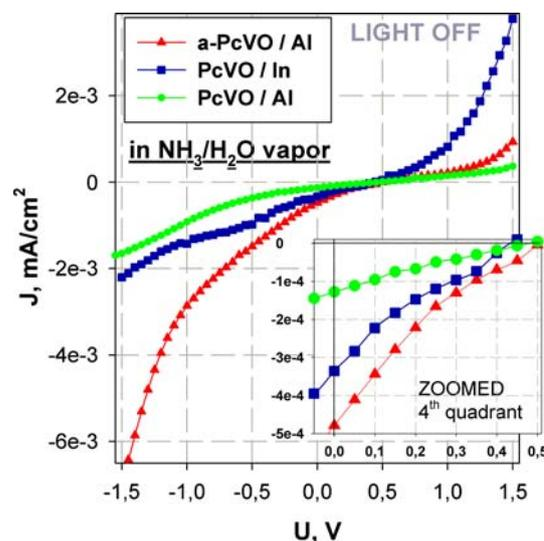
**Fig. 2**  $J$ – $V$  plots for the cells with a 200-nm thick PcVO layer and Al or In cathode, and with less crystalline (denoted as a-PcVO) layer [14], measured in the NH<sub>3</sub> + H<sub>2</sub>O vapor in the dark
