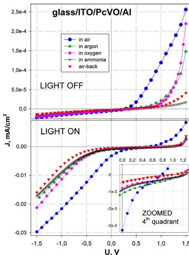
**Fig. 1** Dark and light  $J$ - $V$  plots for the cells with a 200-nm thick crystalline PcVO layer measured in different atmospheres (top-to-down sequence) and back in air at room temperature. Forward bias corresponds to the positively charged ITO electrode
